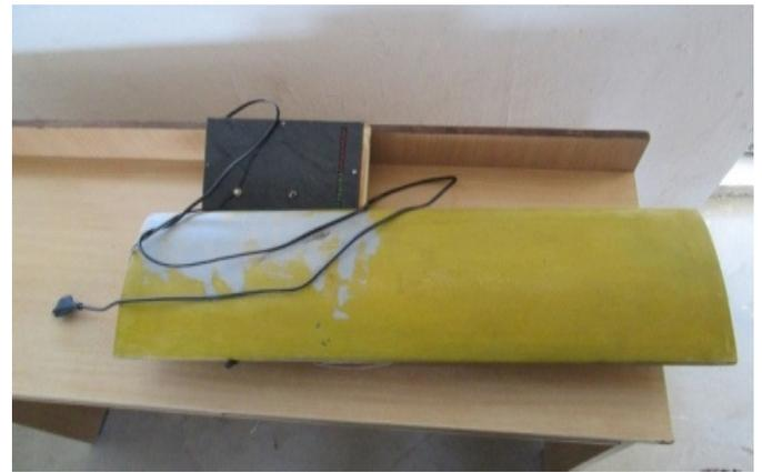
Figure 7. Real Time Model with Piezoelectric Actuator
